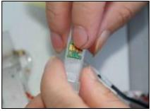
Then stick original chips according to color of cartridges. Please make sure that the chips number matches cartridge number.
